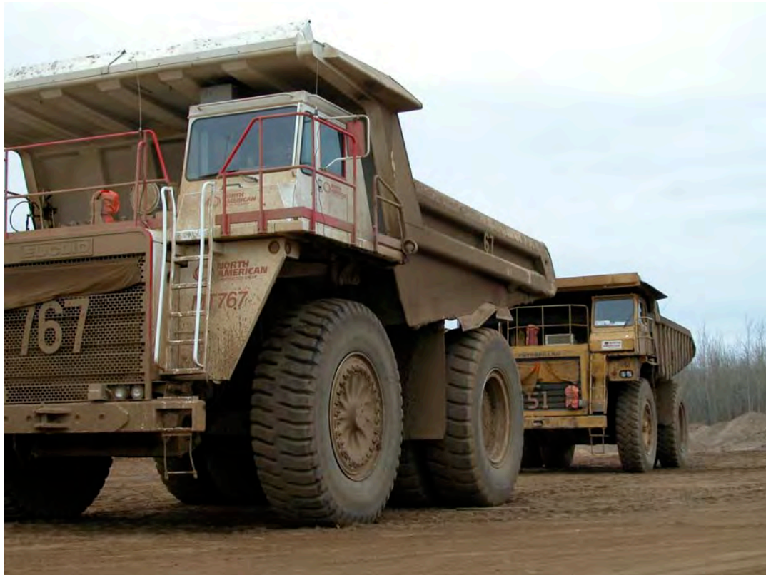
Large trucks used for mining are the primary source of NO x emissions in the oilsands
