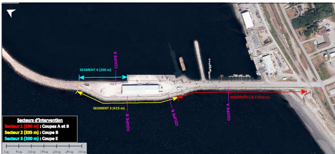
Figure 2-1: Segments of the west breakwater targeted for complete elevation (taken from Lasalle | NHC, 2024)
