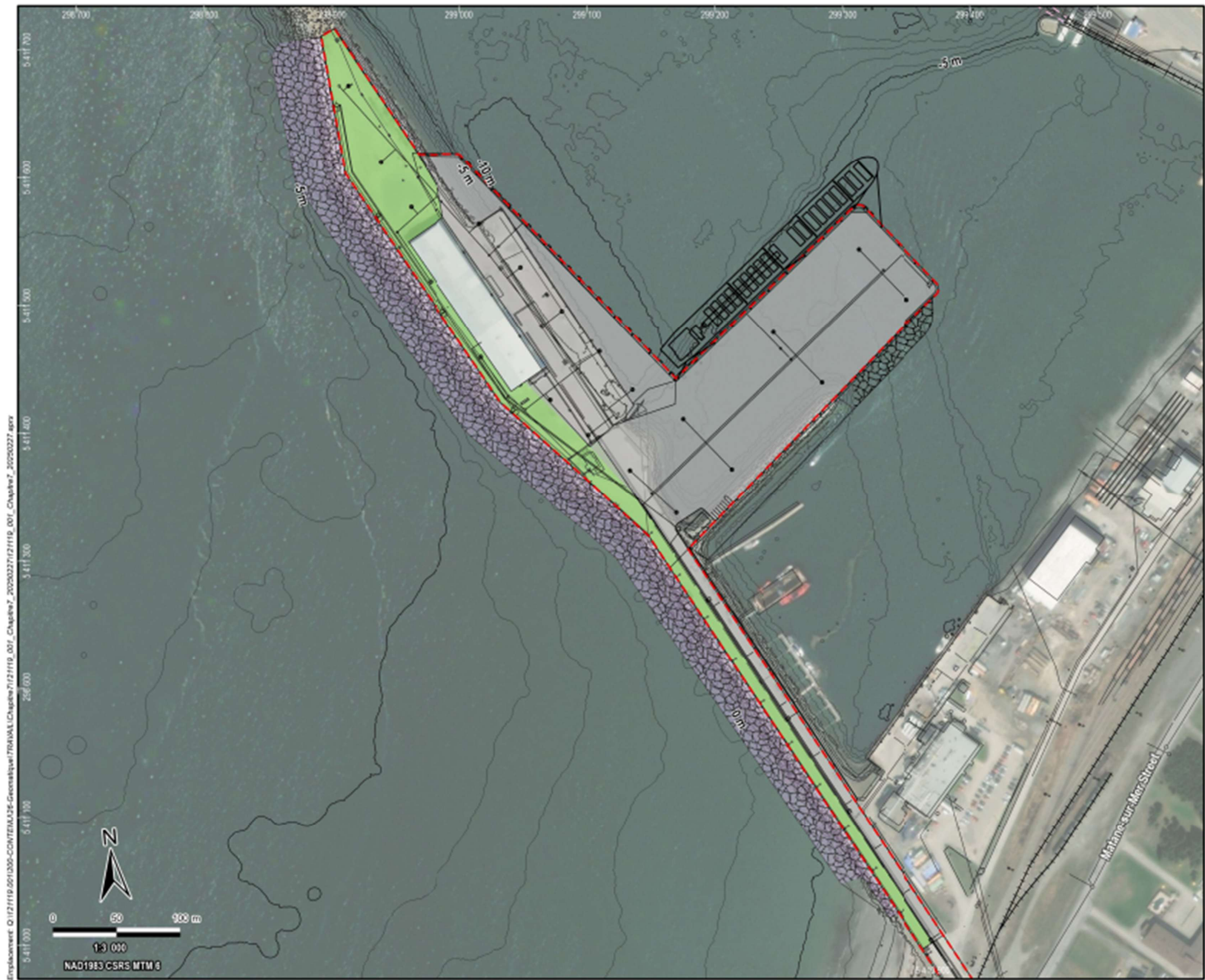
Map 2-7: Representation of Phase 5 (Development of Handling and Storage Areas and Elevation of the West Breakwater)
