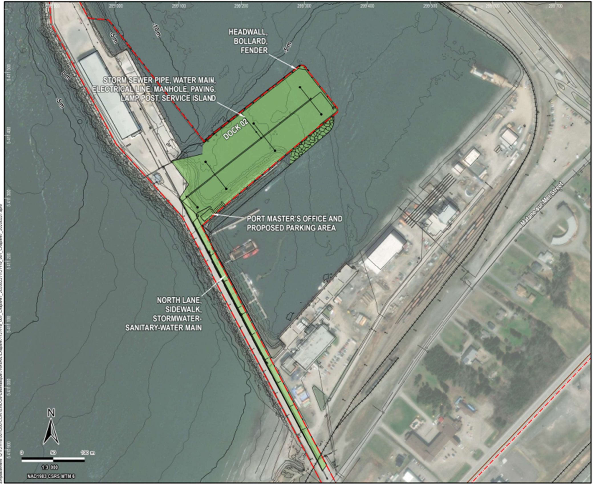
Map 2-5: Representation of Phase 3 (Construction of Berth No. 2 and Installation of Service Systems)
