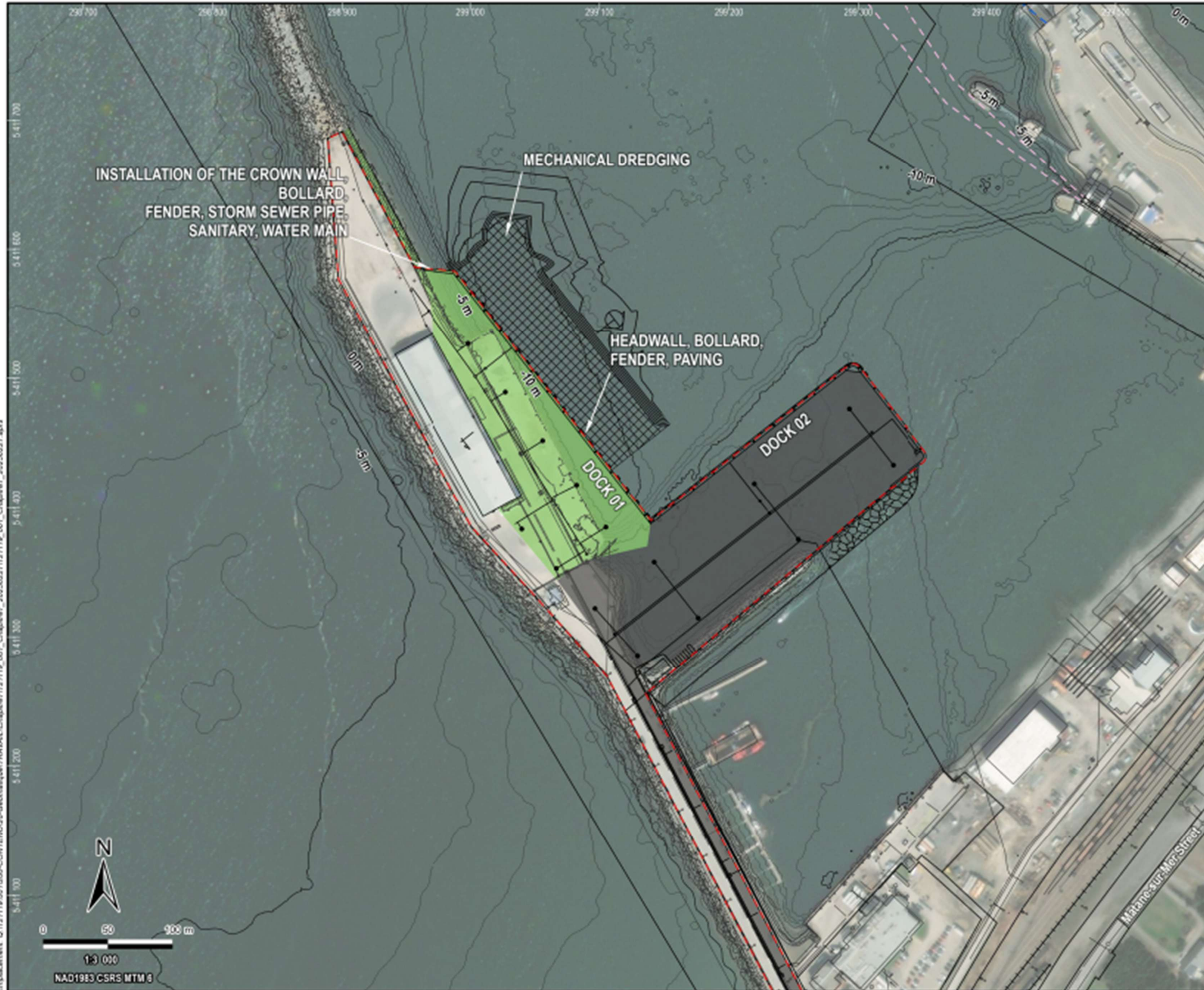
Map 2-6: Representation of the Phase 4 (Mechanical Dredging, Demolition and Reconstruction of Berth No. 1)
