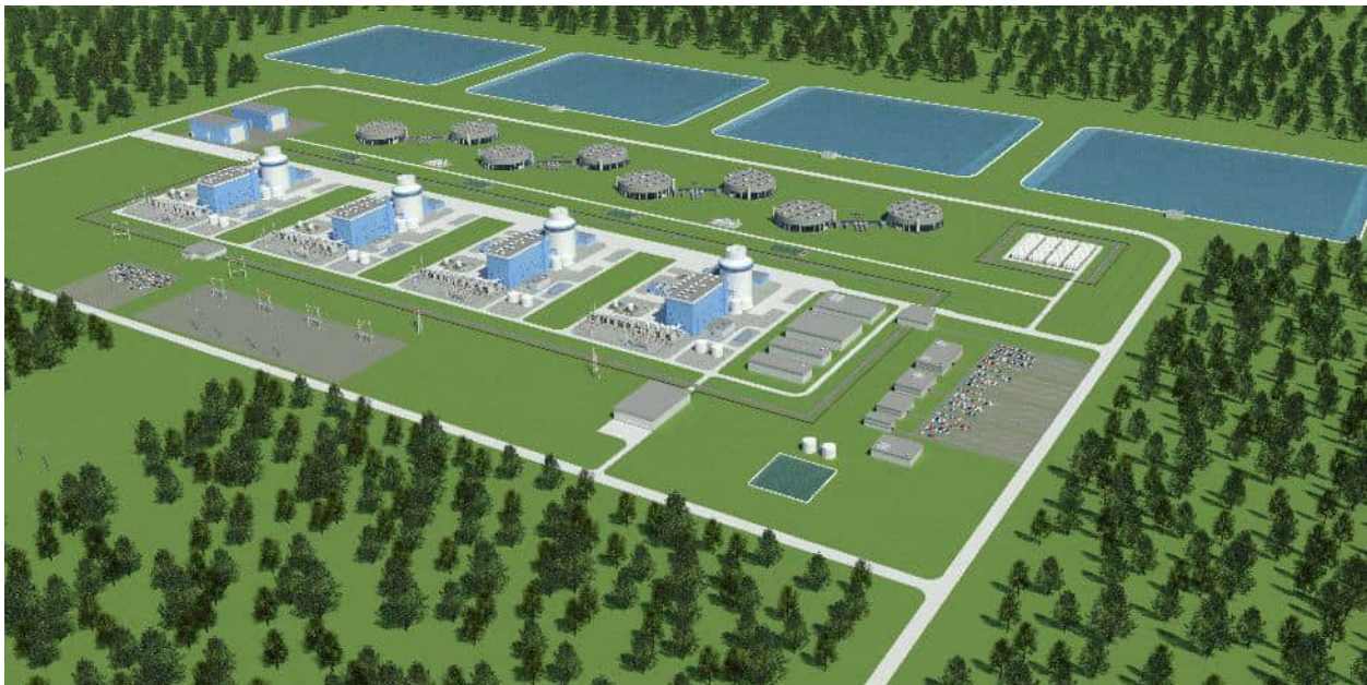
Figure 4.4-9: Conceptual Site Cooling Water Infrastructure Diagram for AP1000 Option
