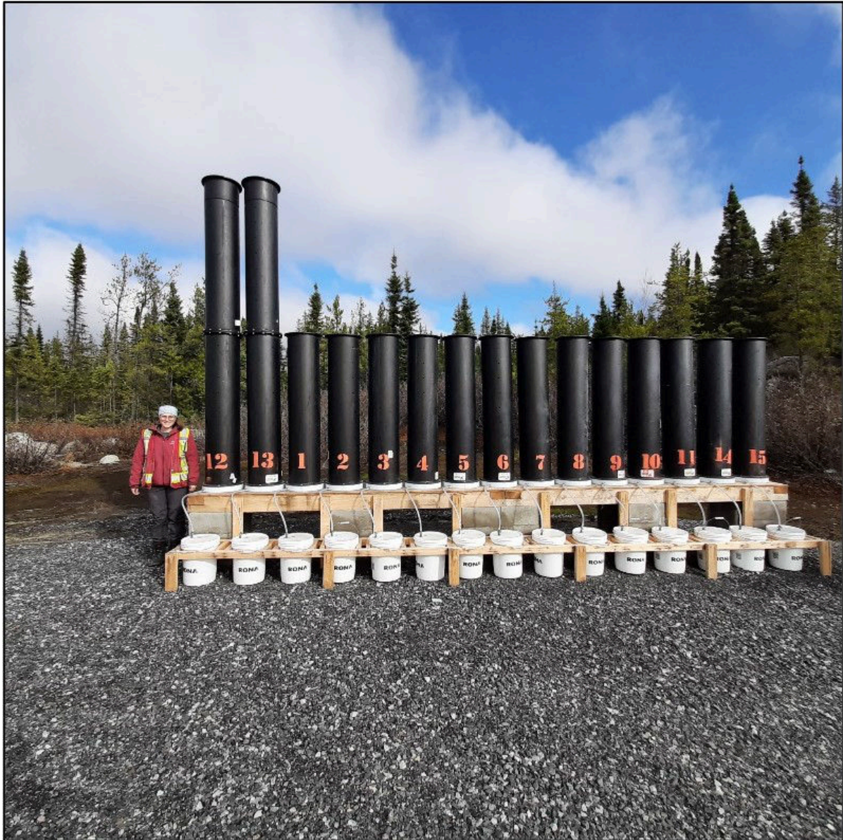
Figure 6-18. A photograph of the 13 on-site ML-ARD columns, with Columns 12 and 13 containing hundreds of kg of existing, weathered J4 waste rock.
