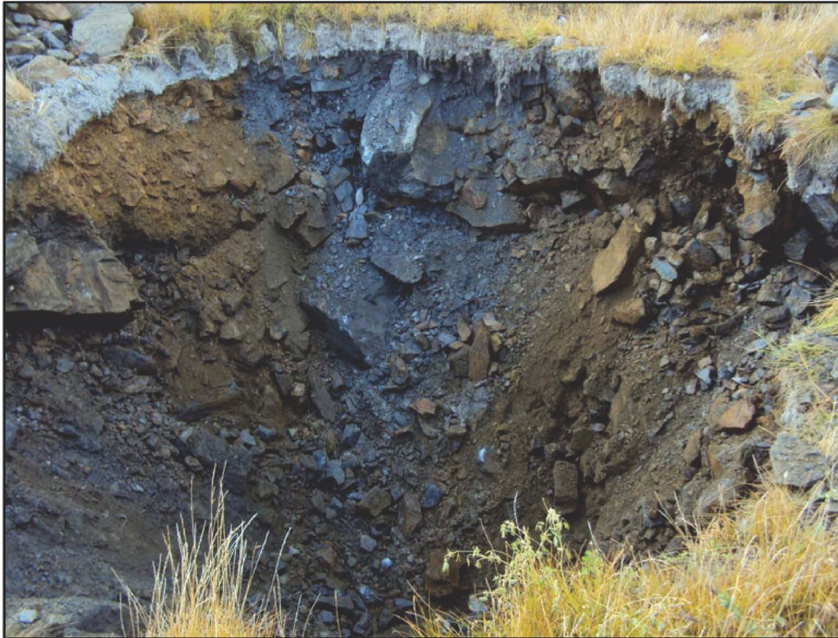
Figure 6-19. A photograph of J4 Test Pit M4 by SRK (2011) showing the type of rock filled into Column 12 including abundant fine-grained particles.
