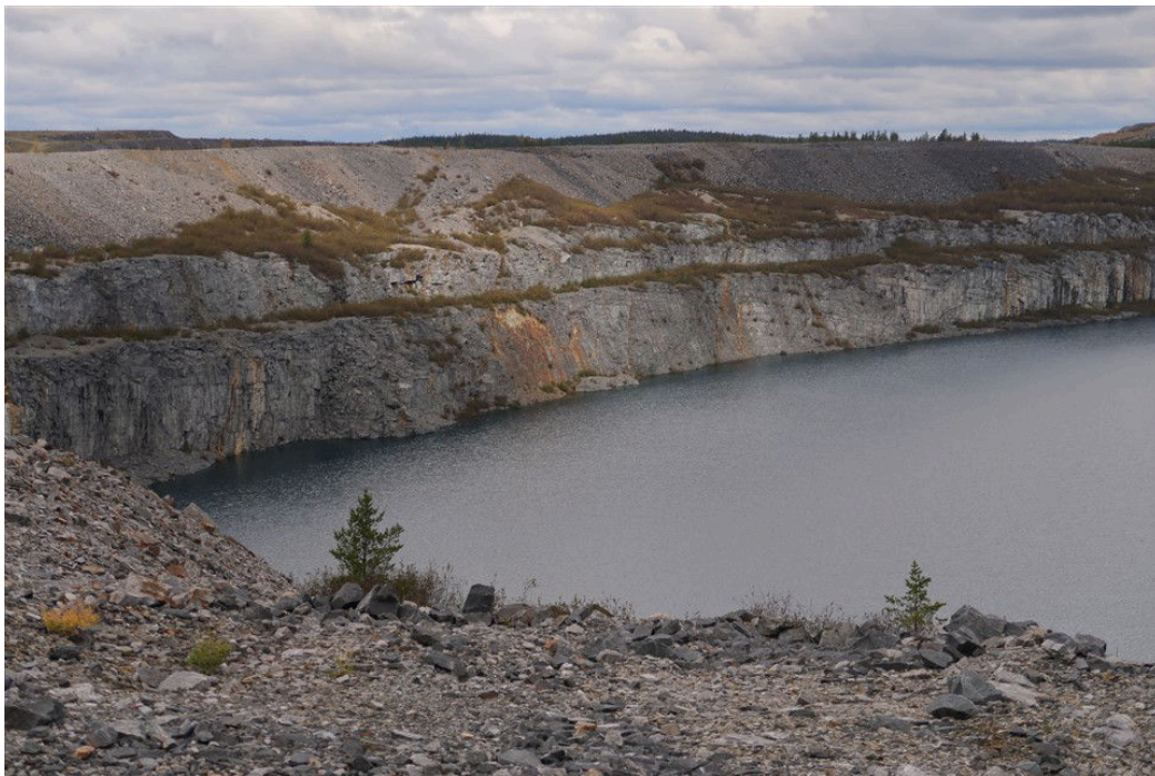
Figure 6-21. Photographs of Troilus waste rock (top) and pit walls (bottom), showing the visible difference between brown oxidized rock and grey unoxidized rock, also seen in Figures 6-19 and 6-20 (photos from the National Research Council of Canada, October 2023).
