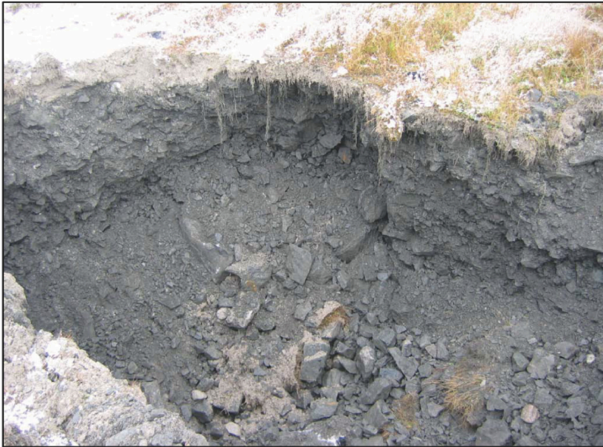
Figure 6-20. A photograph of J4 Test Pit SW5 by SRK (2011) showing the type of rock filled into Column 13 including abundant fine-grained particles.
