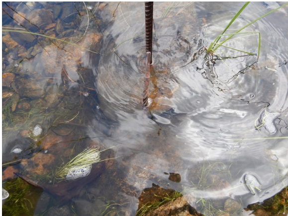
Figure 46: Survey or boundary markers of rebar (rear) and old drill bit (foreground)
