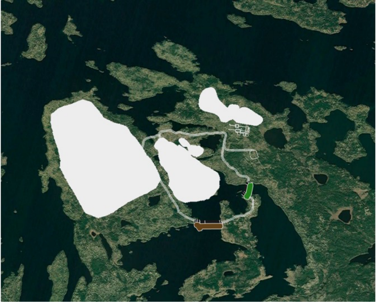
Map 4: Proposed layout of the Springpole Gold Project. The white polygons represent, from left to right, mine rock storage, open pit and stockpiles, process plant and waste rock storage. The map also shows the location of two coffer dams (brown and green), and mine road (source: First Mining Gold).
